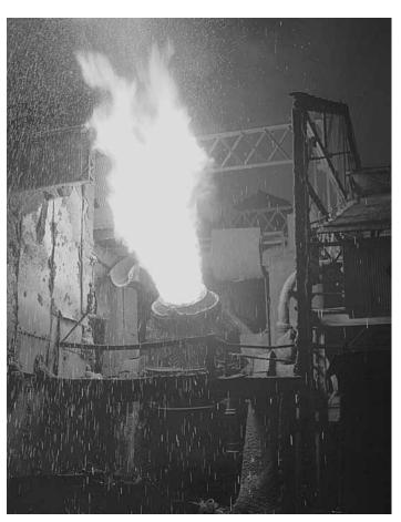
Molten iron is blown in an Eastern Bessemer converter to change it to steel at Republic Steel in Youngstown, Ohio, 1941.
